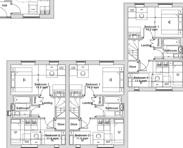
PLOTS 4-6 - BR-LOXLEY 2b4p House Plots 4 & 6 - 79.0 sqm (GIFA) Plot 5 - 78.8 sqm (GIFA) First Floor Plan
