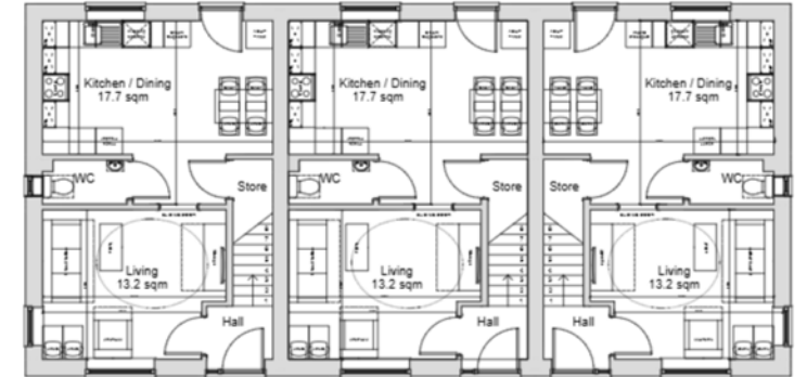
PLOTS 1-3 - BR-LOXLEY 2b4p House Plots 1 & 3 - 79.0 sqm (GIFA) Plot 2 - 81.8 sqm (GIFA) Ground Floor Plan
